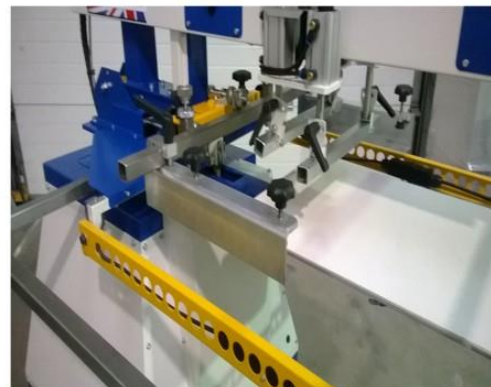
Above PLC touch screen controller allows easy access to the machine functions. This is a very easy to use system and can be learned to operate in a few minutes. The picture on the right shows micro adjustment and frame loading clamps.
