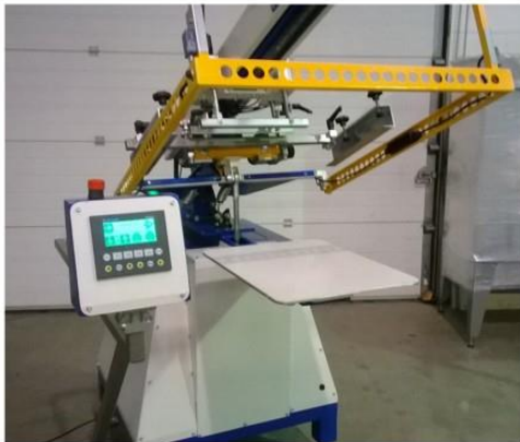
Above PLC touch screen controller allows easy access to the machine functions. This is a very easy to use system and can be learned to operate in a few minutes. The picture on the right shows micro adjustment and frame loading clamps.
