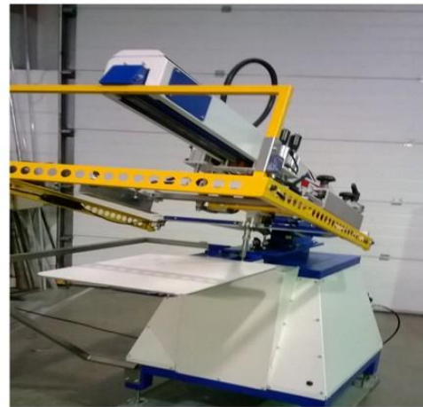
Above shown with standard rubber coated pallet for textile products. Yellow safety guards prevents operator injuries, if the guard is tripped the head gently rises away from the operator.
